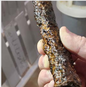
Carbon steel test 30 days
