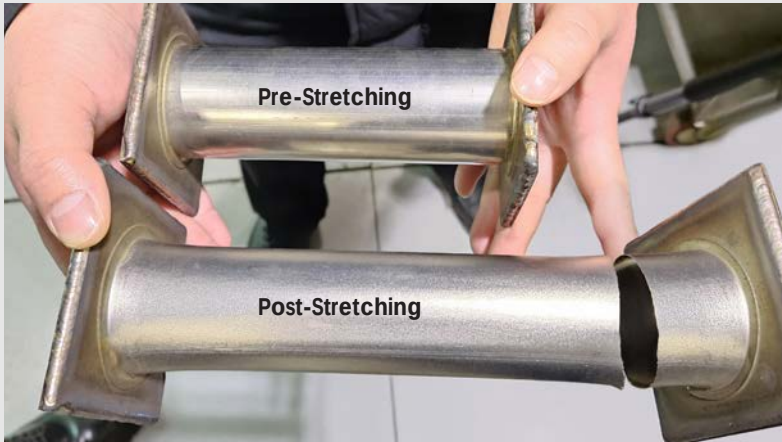
Stainless Steel Core Tube Fracture Test
