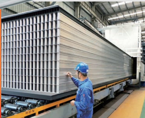
Hot-wind copper brazing oven. It can process 240 m 2 of core slabs brazing in each batch, each chamber can output 12 batches per day
